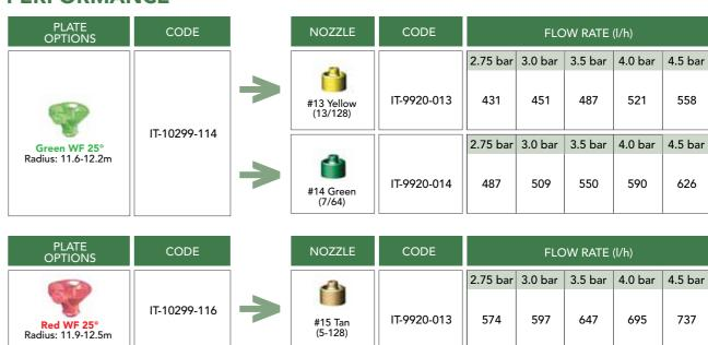
The performance data in this section has been recorded under ideal test conditions and may be adversely affected by poor hydraulic entrance conditions, slope, riser tilt, temperature, wind or other factors.
